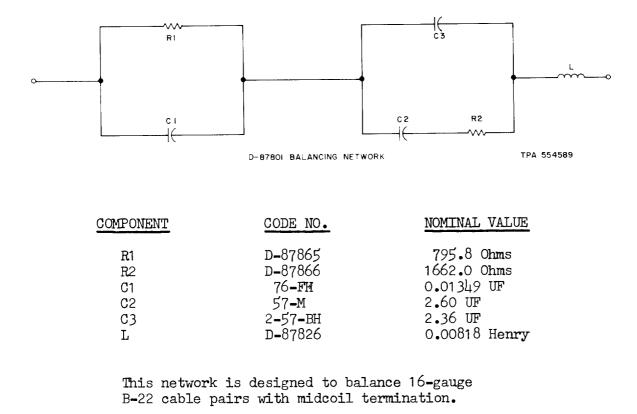
Fig. 1-2-Wire Circuits Employing 16-GA B-22 Cable Pairs-Schematic of Balancing Network
