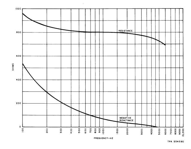
Fig. 2—Impedance Characteristic of D-87801 Balancing Network—This Network is Designed to Balance 16-GA B-22 Cable With Midcoil Termination
