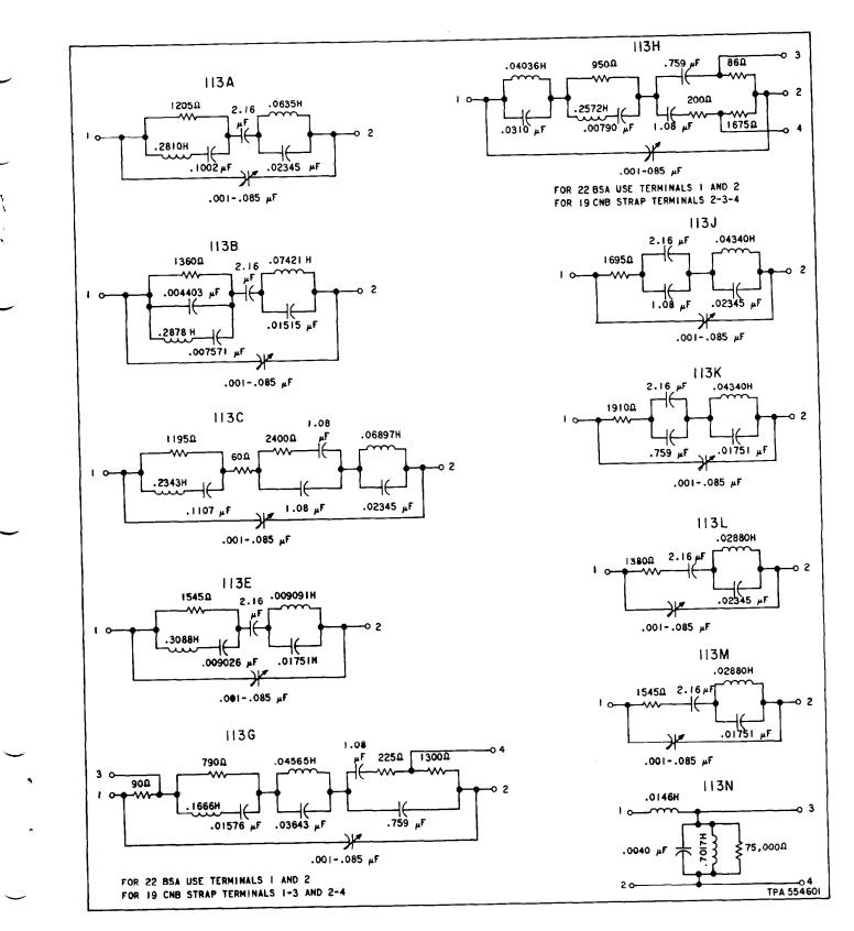
Fig. 2—113-Type Networks for Exchange Facilities
