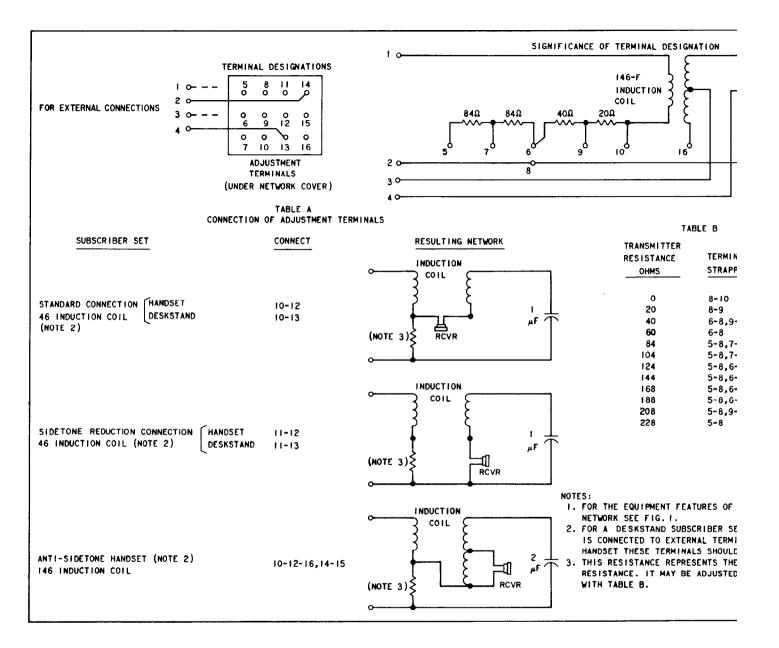
Fig. 4—113F Balancing Network for Subscriber Sets
