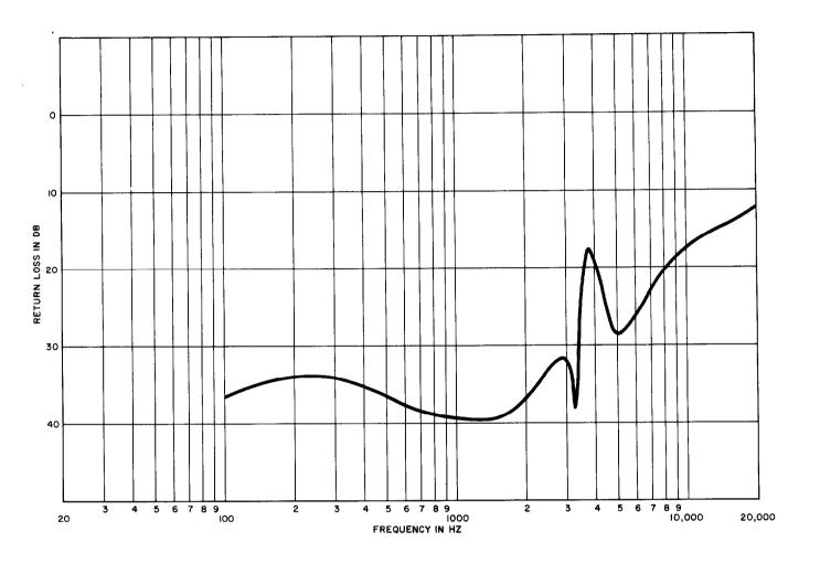
Fig. 4 — 4066B Network — Return Loss vs 26H88 Cable — End Section = 0.50 Loading Section
