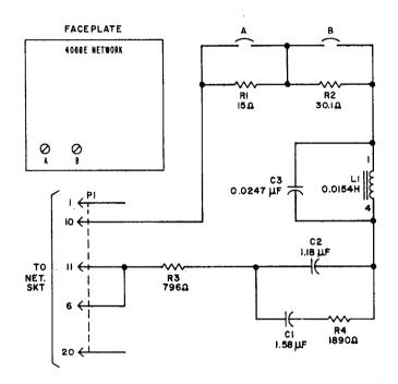
Fig. 2 — 4066E Network — Schematic
