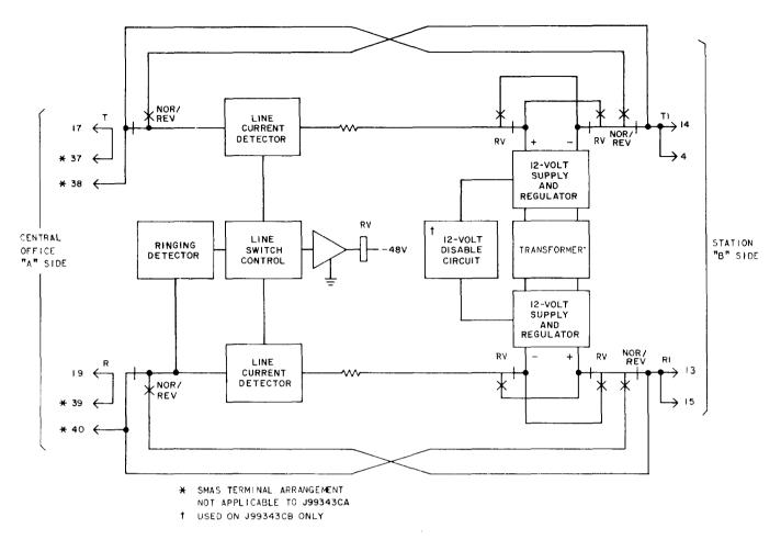
Fig. 4—Block Diagram of the J99343CA, CB, and CC Loop Signaling Extender
