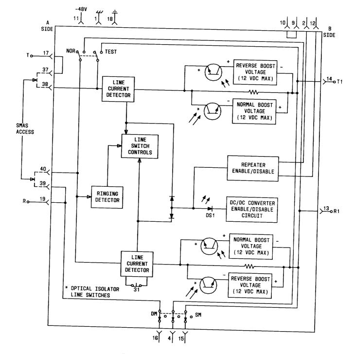
Fig. 11—Block Diagram of the LSE II
