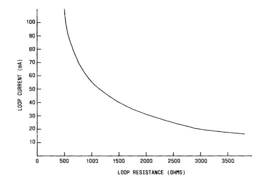
Fig. 15-J99343CE Loop Current Regulating Characteristics
