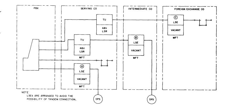
Fig. 8—Typical Application of the LSE in an Off-Premises Station A & B and Foreign Exchange Trunk C
