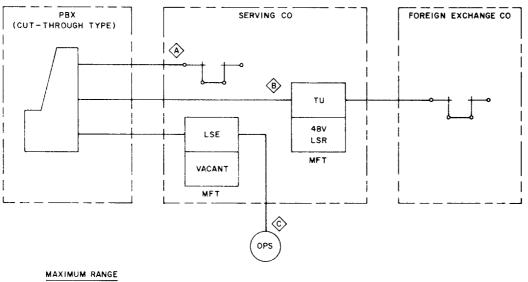
$\langle A \rangle$  TO  $\langle C \rangle$  = PBX TRUNK PLUS STATION LIMIT (NOT TO EXCEED 2400 OHMS).  $\langle B \rangle$  TO  $\langle C \rangle$  = LSR RANGE (NOT TO EXCEED 2400 OHMS).
