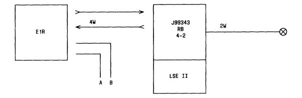
Fig. 12—Typical Application Requiring Ring-Trip boost When Ringing Originates on B-side
