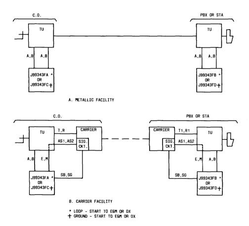
Fig. 1—Metallic and Carrier Applications of the J99343FA, FB, FC, FD Signaling Converters
