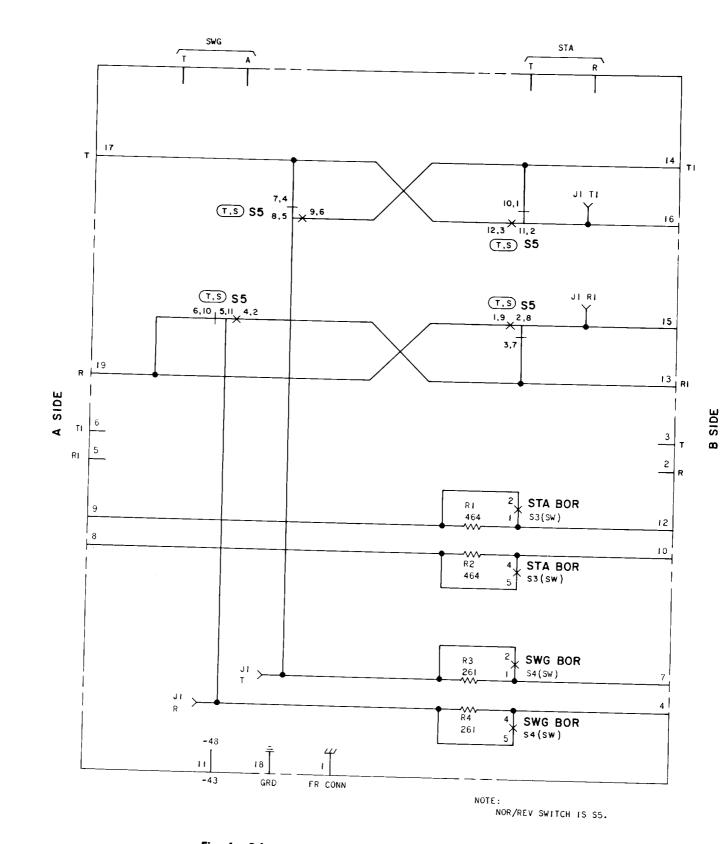
Fig. 4—Schematic of J99343BB Bypass Transmission Unit
