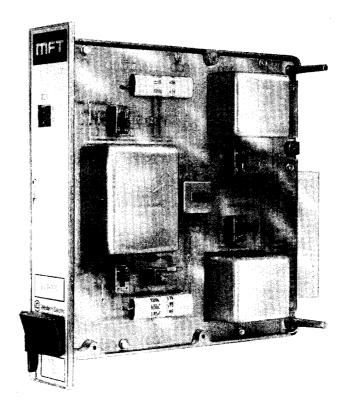
Fig. 5—Two-Wire Transmission Unit J99343BC
