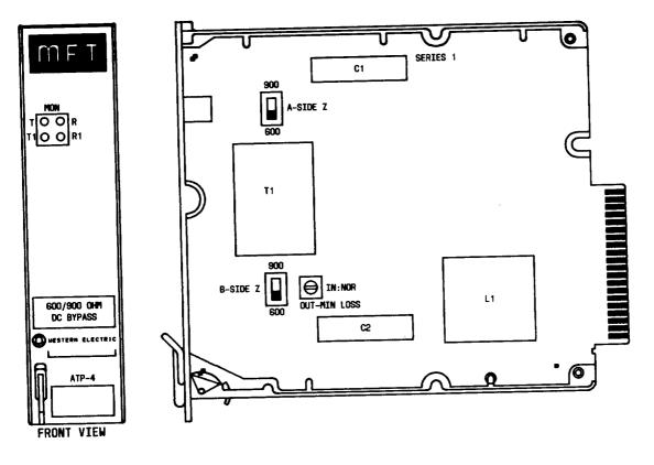
♦Fig. 7—ATP-4 600/900 dc Bypass Unit ♦
