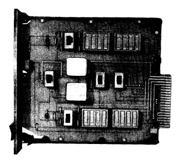
Fig. 2—J99343BD 4-4 Wire Transmission Unit Controls
