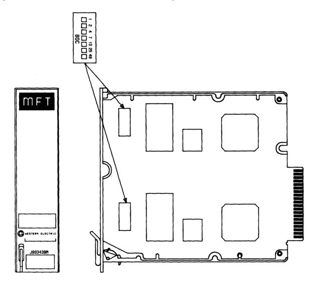
Fig. 3—Component Layout, J99343BM
