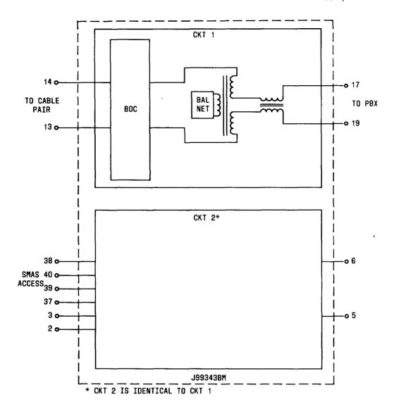
Fig. 4-Block Diagram, J99343BM
