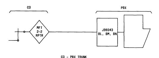
Fig. 7—Typical Application of Impedance Compensation Network
