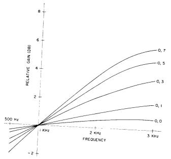
Fig. 10—Amplifier/Equalizer Response A=0
