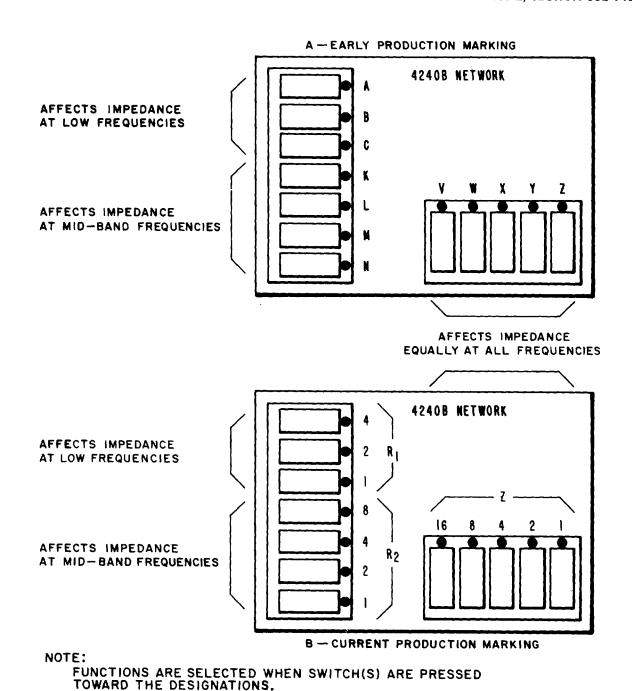
Fig. 4—Precision Balance Switch Functions J99343PB, L1, L2
