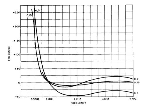
Fig. 12—Envelope Delay Distortion C=0
