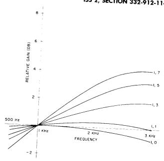
Fig. 11—Amplifier/Equalizer Response A=1
