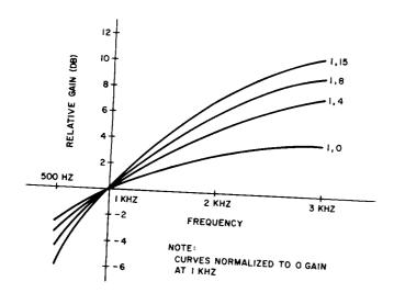
Fig. 9—Amplifier/Equalizer Response C=1
