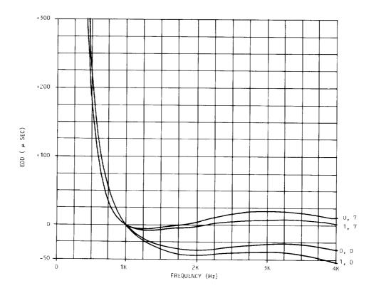
Fig. 14—Envelope Delay Distortion, J99343PB, L3
