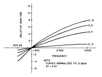
Fig. 8—Amplifier/Equalizer Response C=0
