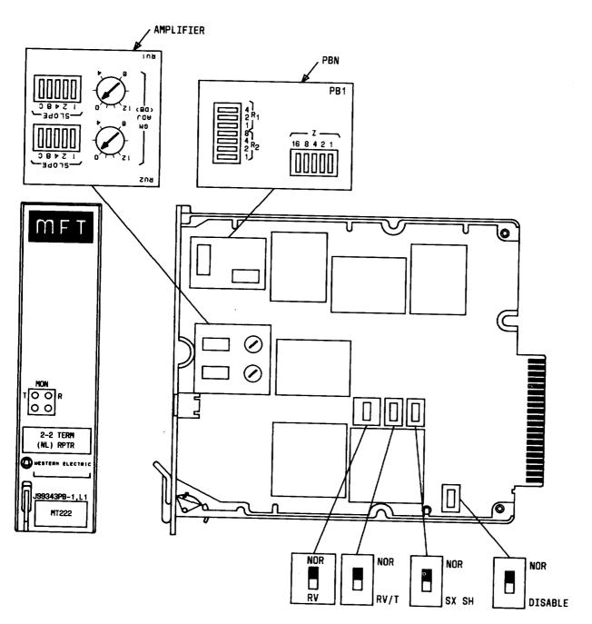
Fig. 1—Component Layout, J99343PB, L1
