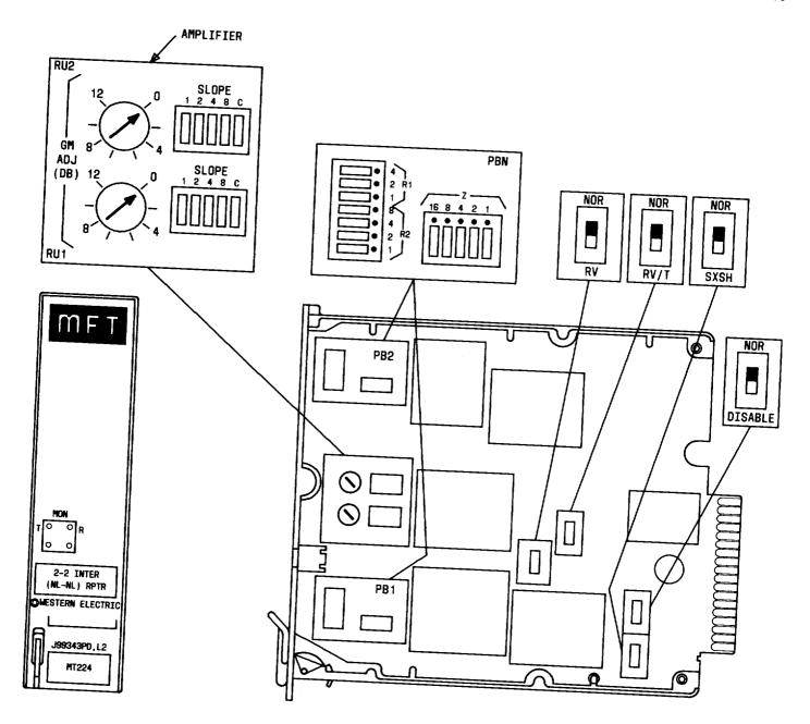
Fig. 2—2-2 Intermediate (NL-NL) Repeater J99343PD, L2 (MD) Component Layout
