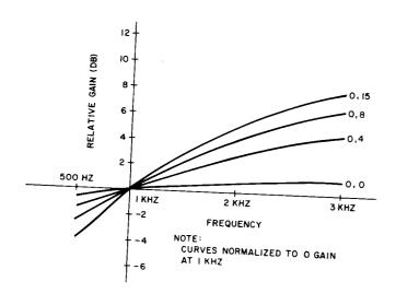
Fig. 8—Amplifier/Equalizer Frequency Response of the 309D Amplifier Unit—C Switch = O (off)
