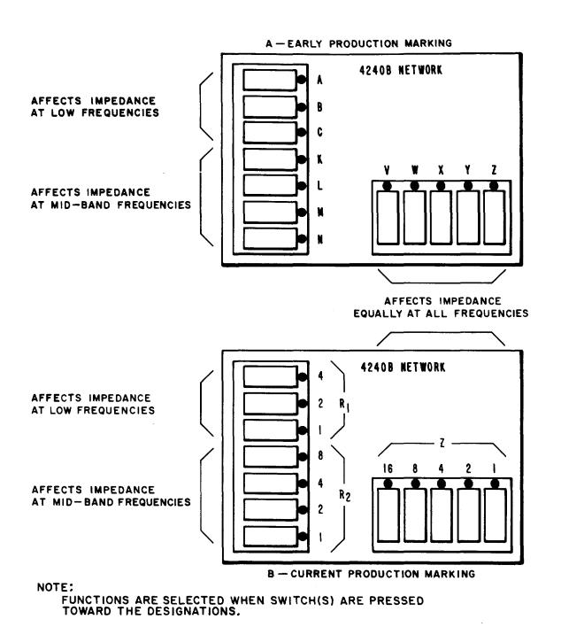
Fig. 4—J99343PD, L1 and L2 Precision Balancing Network Switch Functions
