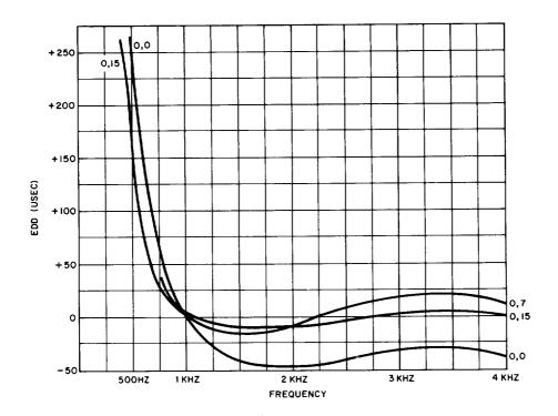
Fig. 10—Envelope Delay Distortion, C = O
