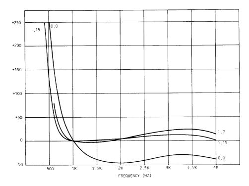
Fig. 11—Envelope Delay Distortion, C = 1
