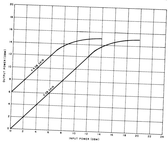
Fig. 12—Output Power Capability of the J99343PD
