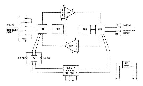
Fig. 7—Block Diagram of the 2-2 Intermediate (NL-NL) Repeater J99343PD,L3
