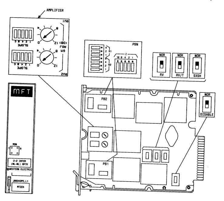
Fig. 1—2-2 Intermediate (NL-NL) Repeater J99343PD, L1 (MD) Component Layout
