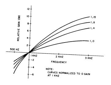
Fig. 9—Amplifier/Equalizer Frequency Response of the 309D Amplifier Unit—C Switch = 1 (Operated)
