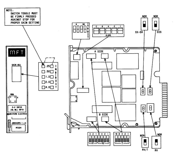
Fig. 6—2-2 Intermediate (NL-NL) Repeater J99343PD, L3 Component Layout
