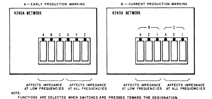
Fig. 4—Control Switches of the J99343PC PBN
