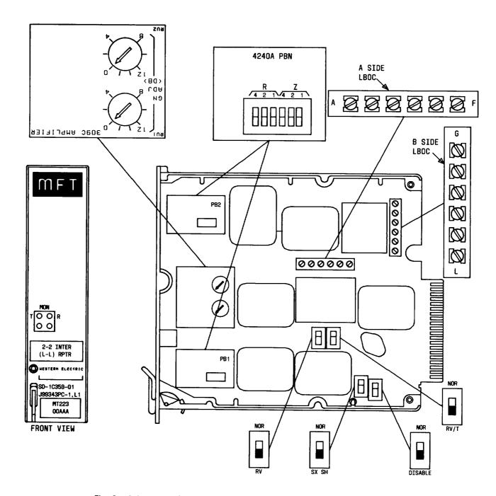
Fig. 1—2-2 Intermediate (L-L) Repeater J99343PC (MD) Component Layout
