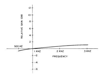
Fig. 9—Amplifier Frequency Response
