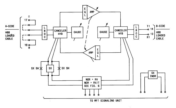
Fig. 8—Block Diagram of the 2-2 Intermediate (L-L) Repeater J99343PH, L2
