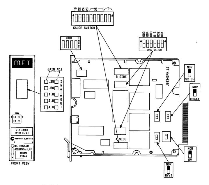
Fig. 7—2-2 Intermediate (L-L) Repeater J99343PH, L2 Component Layout
