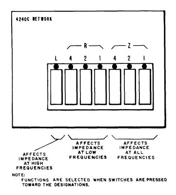
Fig. 5—Control Switches of the J99343PH, L1 PBN
