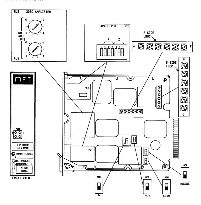
Fig. 2—2-2 Intermediate (L-L) Repeater J99343PH, L1 (MD) Component Layout
