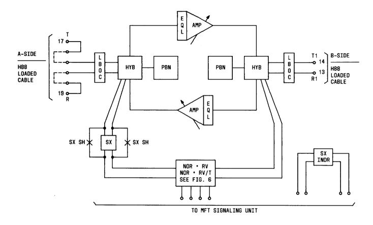
Fig. 3—Block Diagram of the 2-2 Intermediate (L-L) Repeater J99343 PC/PH, L1
