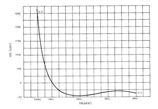
Fig. 10—Envelope Delay Distortion Curve
