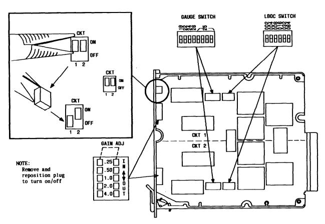
Fig. 3.1—Description of How to Operate the CKT 1,2 (ON/OFF) Plug-Switch of the J99343PL L2 Repeater
