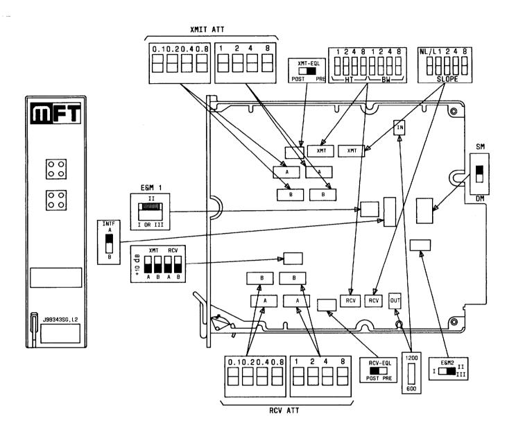
Fig. 3.1—Component Layout of the J99343SG, L2 CFU
