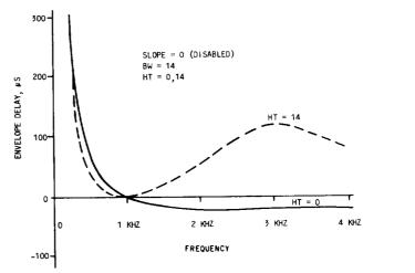
Fig. 15—Relative Envelope Delay Distortion of SF Signaling/4-4 Wire Repeater, BW = Large Setting, HT Variable
