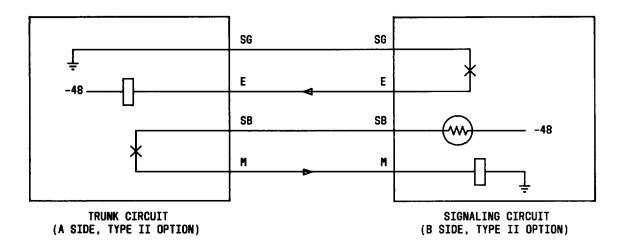
Fig. 6—Type II E and M Interface
