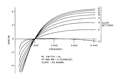
Fig. 8—Gain Frequency Response of the Equalizer Unit, NL/L = L, Slope Variable
