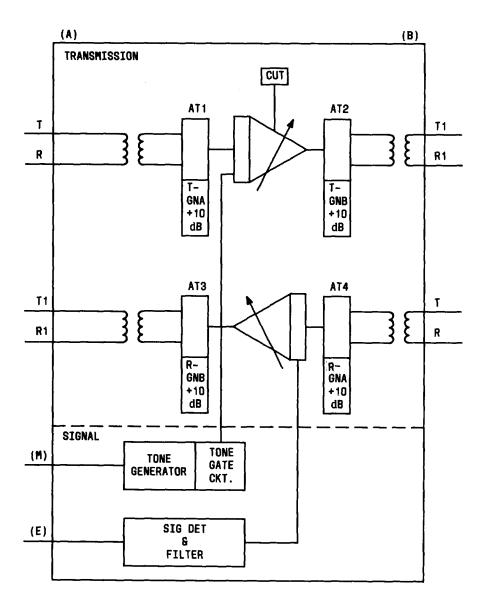
Fig. 2—Block Diagram of the J99343SF CFU
