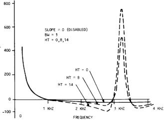
Fig. 14—Relative Envelope Delay Distortion of the SF Signaling/4-4 Wire Repeater, BW = Small Setting, HT Variable
