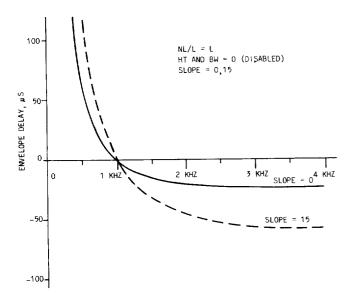
Fig. 13—Relative Envelope Delay Distortion of the SF Signaling/4-4 Wire Repeater, Loaded Cable, Slope Variable
