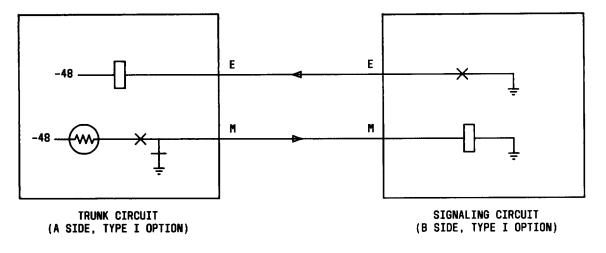
Fig. 5—Type I E and M Interface
