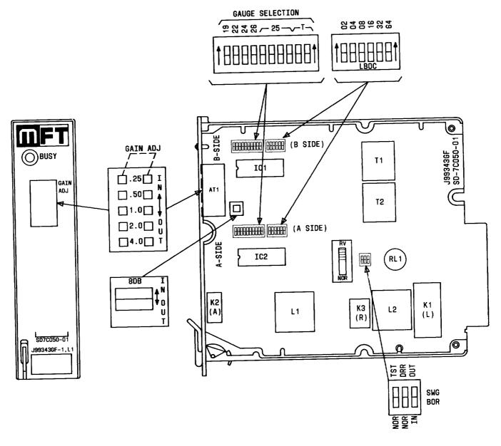
Fig. 1—J99343GF L1—Component Layout
