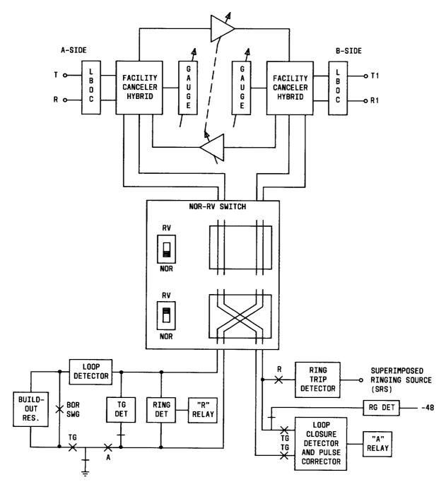
Fig. 5—Block Diagram of J99343GJ CFU♦
