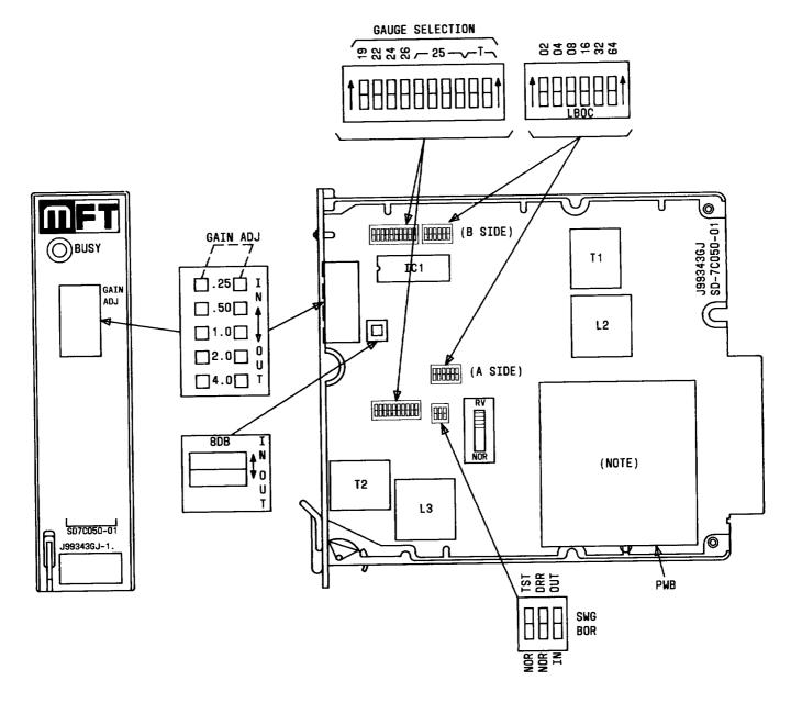
NOTE: DAUGHTER PRINTED WIRING BOARD USING BERGSTIK CONNECTORS CONTAINS GROUND START SIGNALING COMPONENTS OF THE J99343GJ CFU.
