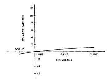
Fig. 6—Amplifier Frequency Response
