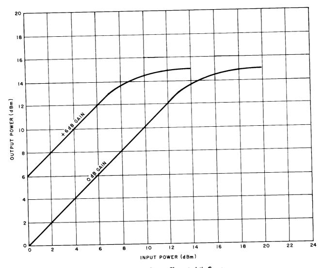
Fig. 8—Output Power Characteristic Curve
