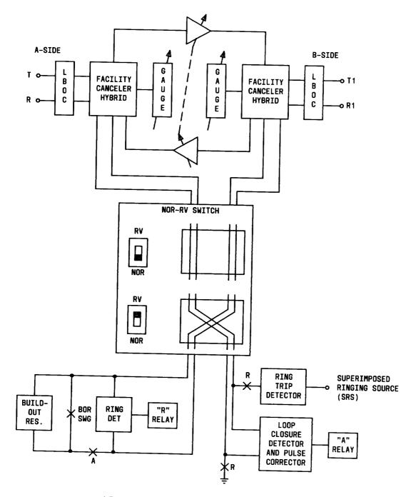
♦ Fig. 2— Block Diagram of the J99343GF (L1&L2) CFUs€
