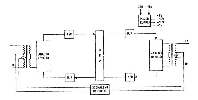
Fig. 1—J99343PR 2-2 Wire Repeater—Block Diagram
