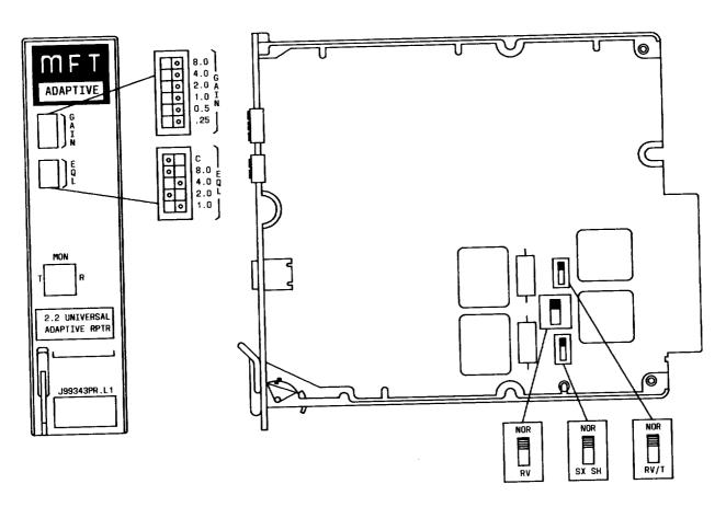
Fig. 2-J99343PR 2-2 Wire Repeater—Component Layout
