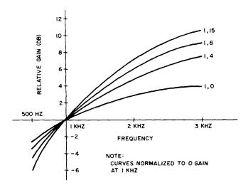
Fig. 5—Amplifier/Equalizer Frequency Response—C
