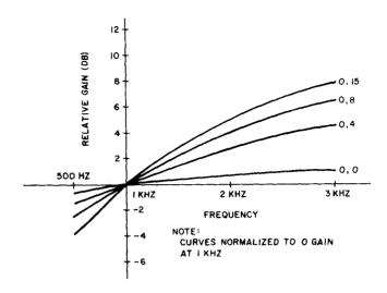
Fig. 4—Amplifier/Equalizer Frequency Response—C
