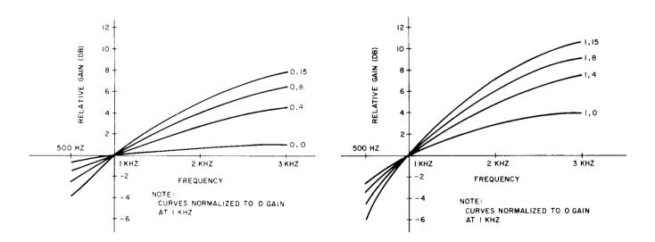
Fig. 3—Equalizer Frequency Response With C=0 (off)
