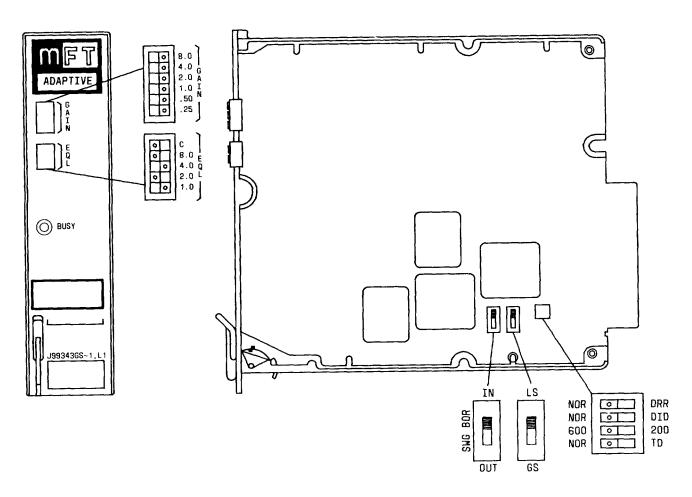
Fig. 1-J99343GS 2-2 Wire CFU-Component Layout
