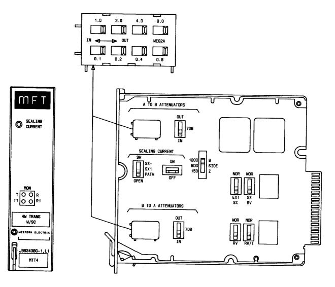
Fig. 1—4-4 Wire Transmission Unit J99343BG Component Layout
