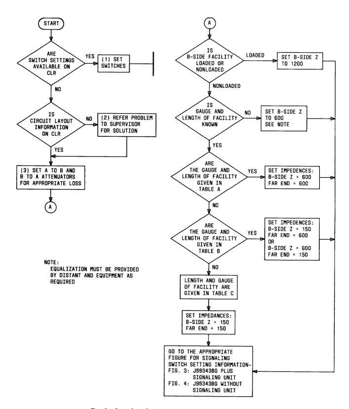
Fig. 2—Procedure for Setting Transmission Controls of J99343BG Unit
