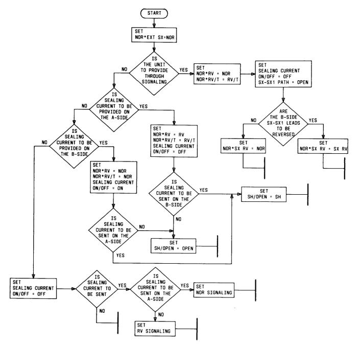
Fig. 4—Signaling Switch Settings for J99343BG Unit Used Without Companion Signaling Unit
