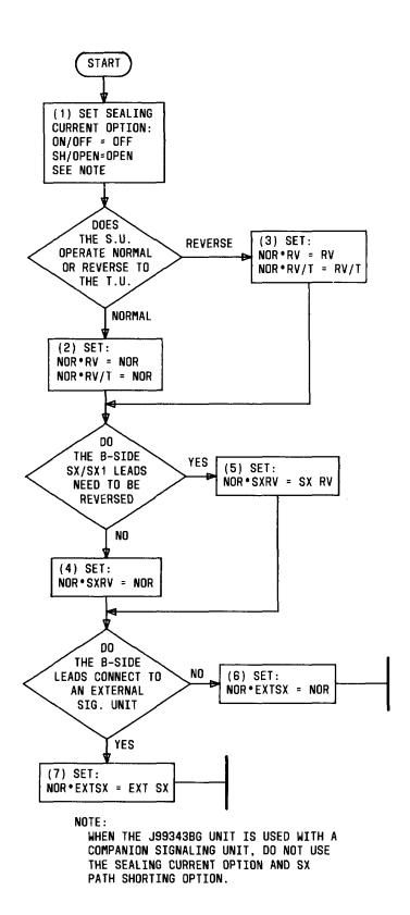
Fig. 3— Signaling Switch Settings for J99343BG Unit Used With Companion Signaling Unit
