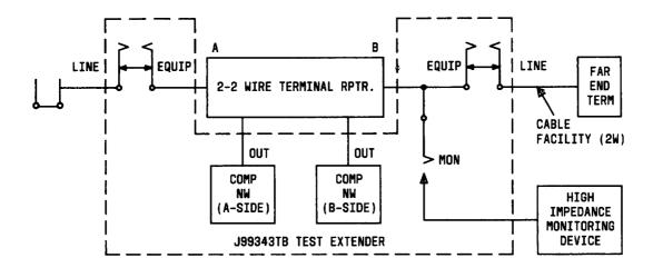
Fig. 12—Typical Circuit Configuration for Stability Margin Tests
