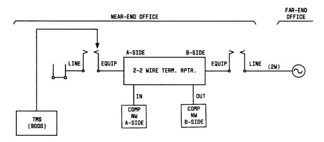
Fig. 10—Typical Test Configuration or Setting A-Side Level Output
