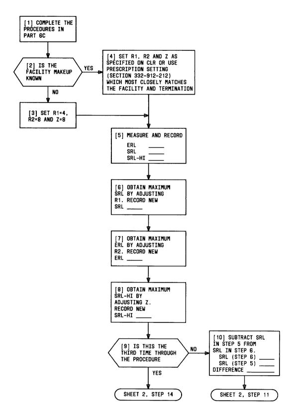
Fig. 5—Procedures for Adjustment of the B-Side PBN (Sheet 1 of 2)
