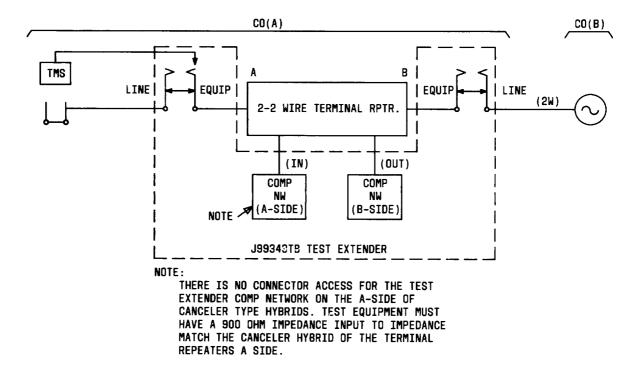
Fig. 7—Typical Test Configuration for Frequency Response Measurements
