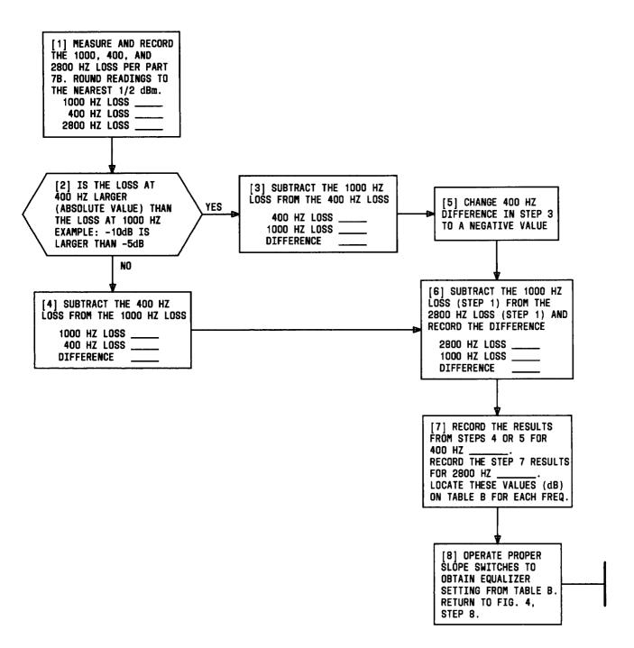
Fig. 8—Obtaining Equalizer Settings by Measurement
