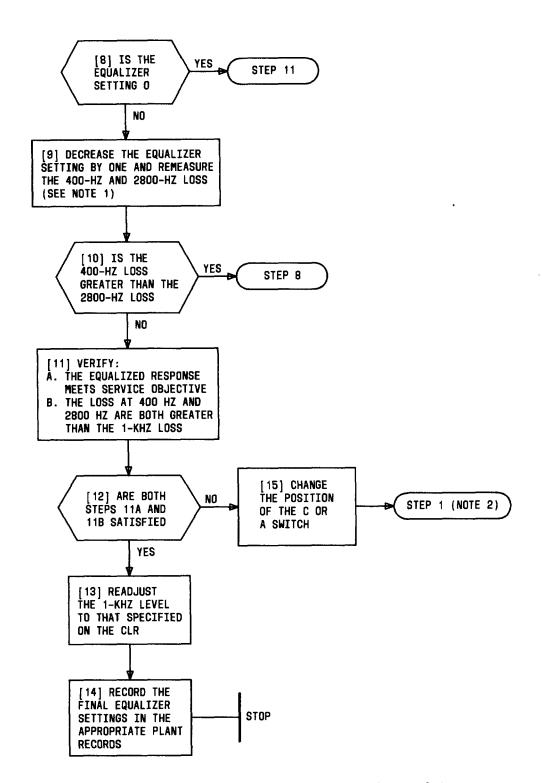
Fig. 11—Procedure for Equalizer Touch-Up (Sheet 2 of 2)
