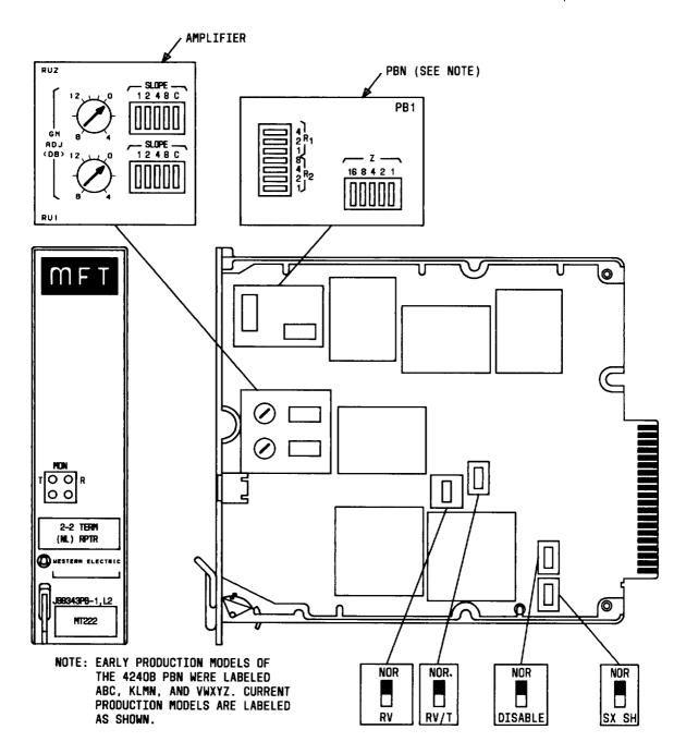
Fig. 2—Component Layout—J99343PB, L2
