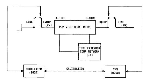
Fig. 9—Test Configuration for Setting Specific Gain
