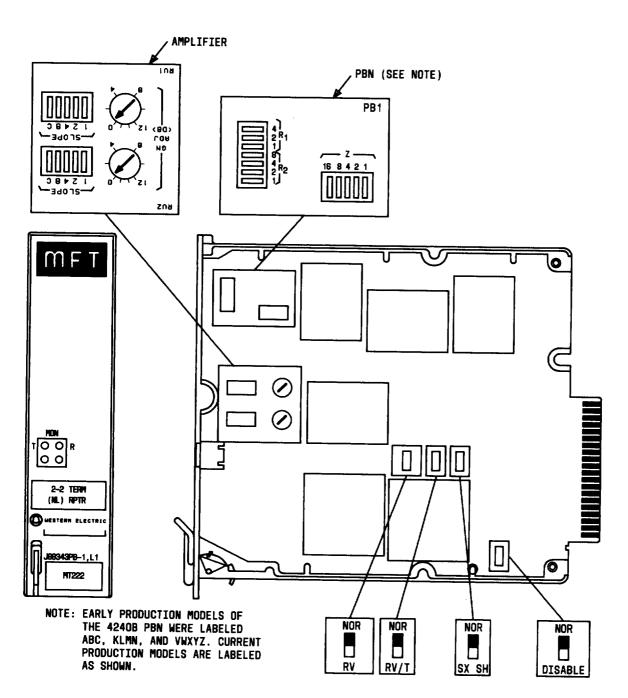
Fig. 1—Component Layout—J99343PB, L1
