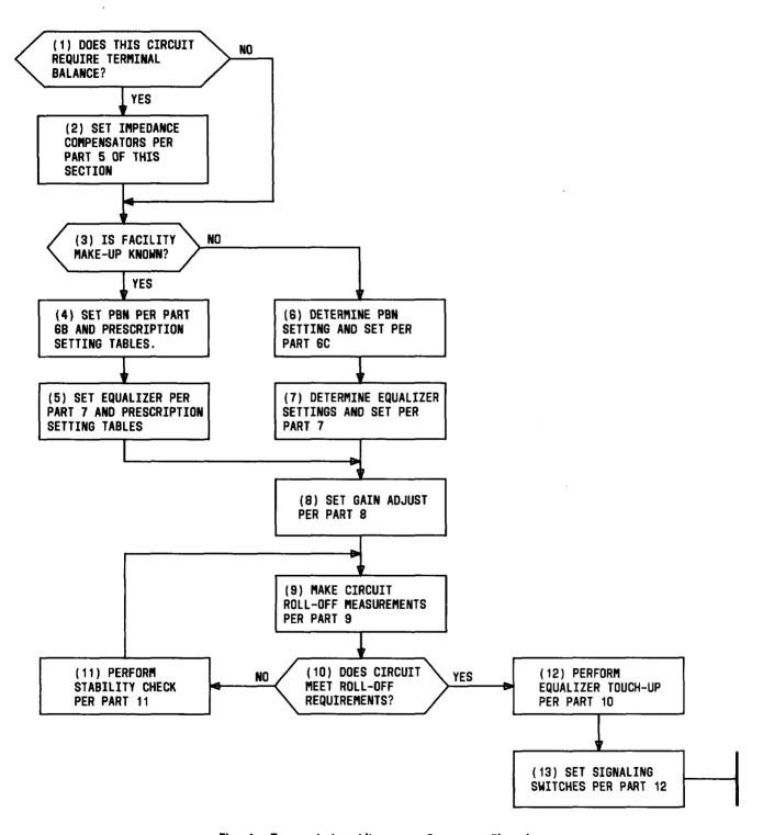
Fig. 4—Transmission Alignment Sequence Flowchart
