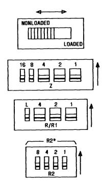
\* R2 SWITCHES ARE NOT USED WHEN BALANCING LOADED CABLE. THESE SWITCHES SHOULD BE OFF.
