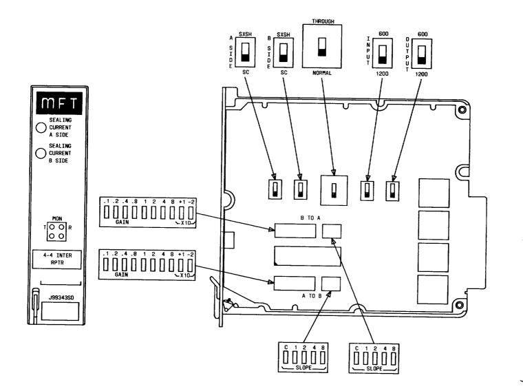
Fig. 2—J99343SD 4-4 Wire Repeater—Switch Layout
