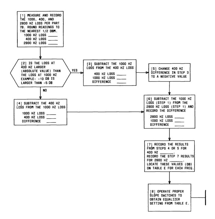
Fig. 9—Obtaining Equalizer Setting By Measurement
