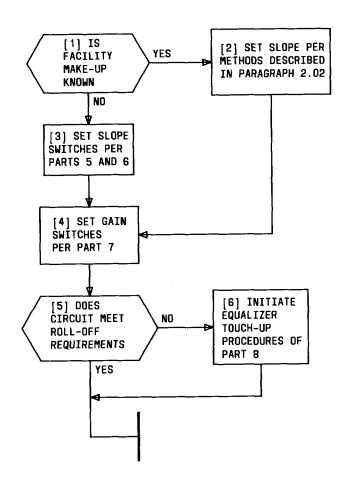
Fig. 4—Transmission Alignment Sequence
