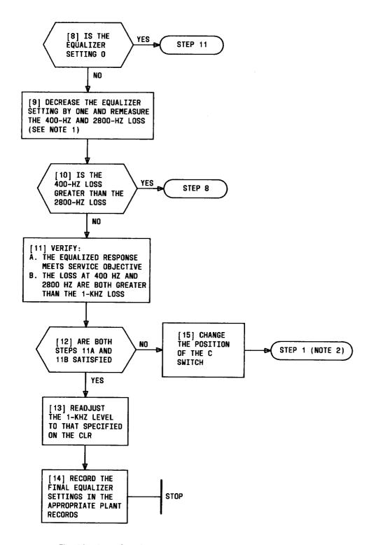
Fig. 10—Procedure for Equalizer Touch-Up (Sheet 2 of 2)
