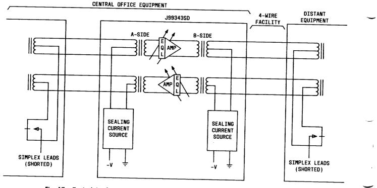
Fig. 17—Typical Application of the J99343SD 4-4 Wire Repeater With Sealing Current
