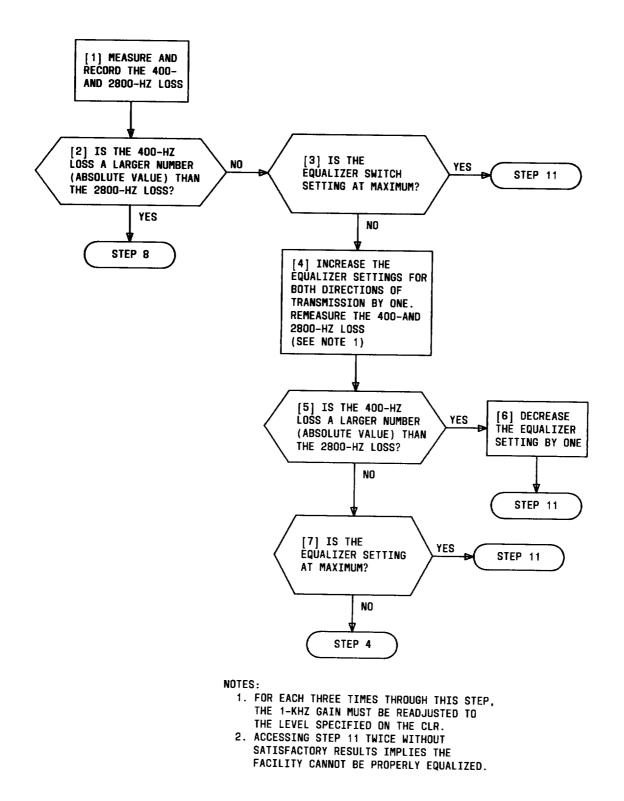
Fig. 10—Procedure for Equalizer Touch-Up (Sheet 1 of 2)
