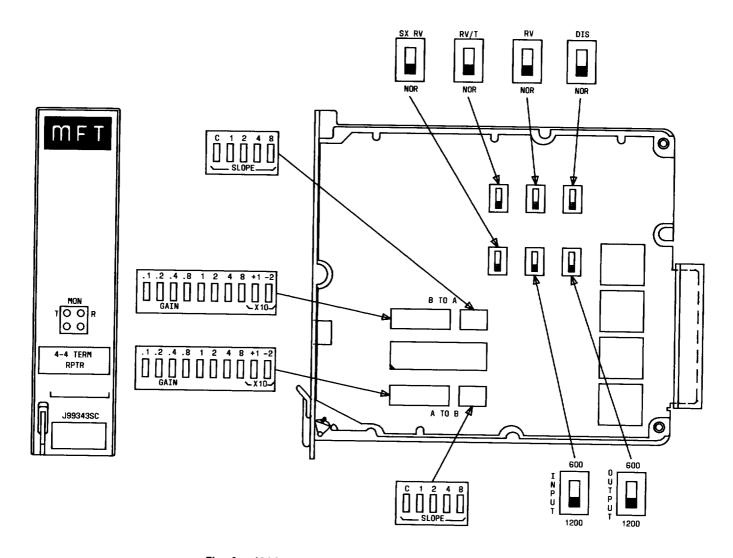
Fig. 1—J99343SC 4-4 Wire Repeater—Switch Layout
