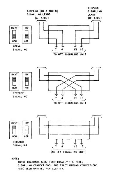
Fig. 11—Signaling Options for the J99343SC Repeater
