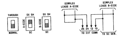
Fig. 14—Switch Settings for SD Repeater to Furnish B-Side Sealing Current
