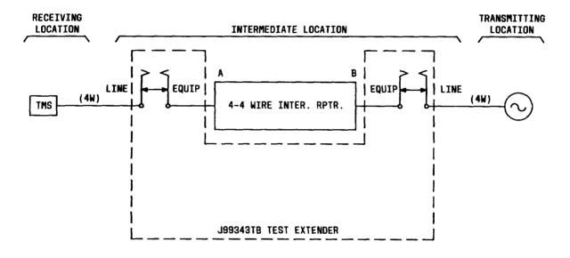
Fig. 8—Typical Test Configuration for Cable Loss Measurement —Intermediate Repeater
