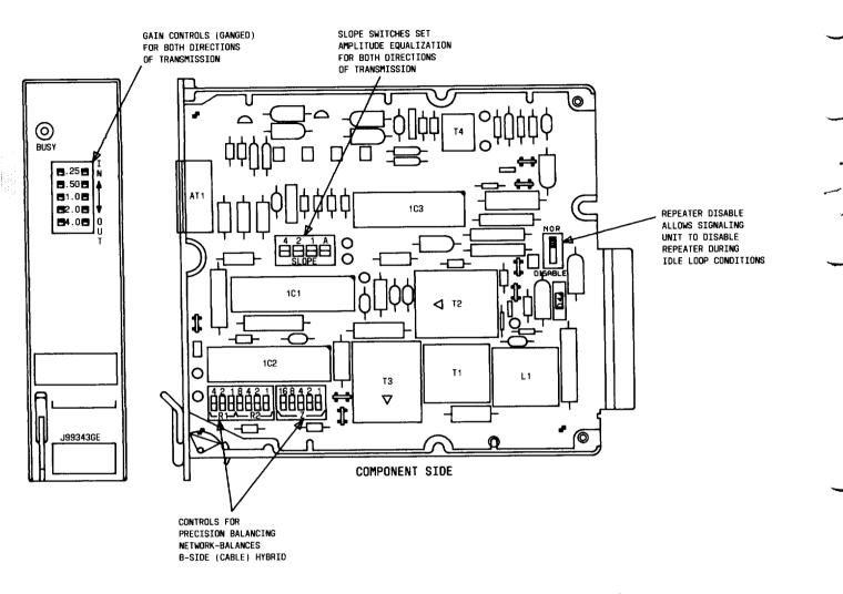
Fig. 1—LSE/2-2 Wire (NL) Terminal Repeater (J99343GE) Component Layout
