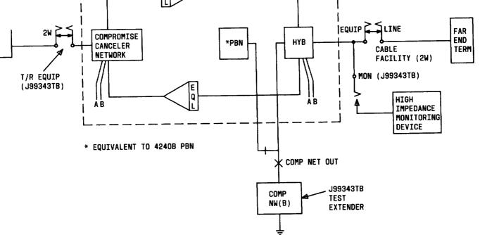
Fig. 5—In-Circuit Configuration for Stability Tests of the J99343GE Combined Function Unit
