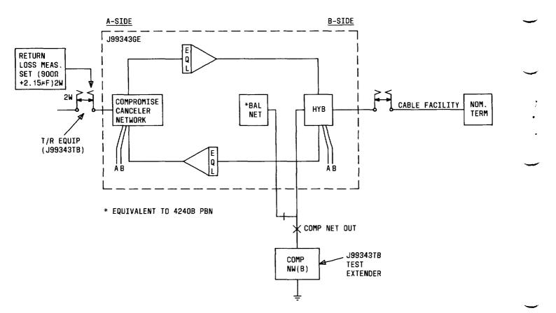
Fig. 3—Test Configuration for Determining IC Balancing Network Settings by Measurement for the J99343GE Combined Function Unit (B-Side)
