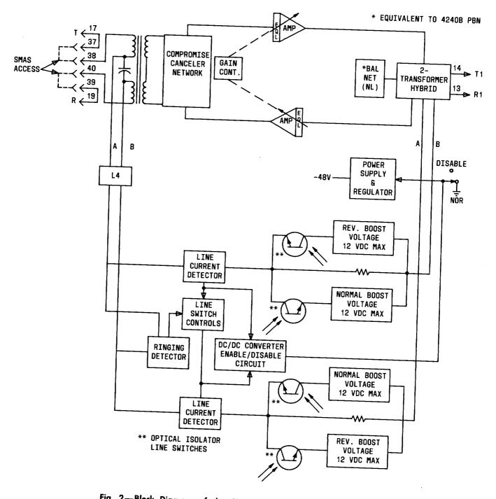
Fig. 2—Block Diagram of the J99343GE Combined Function Unit
