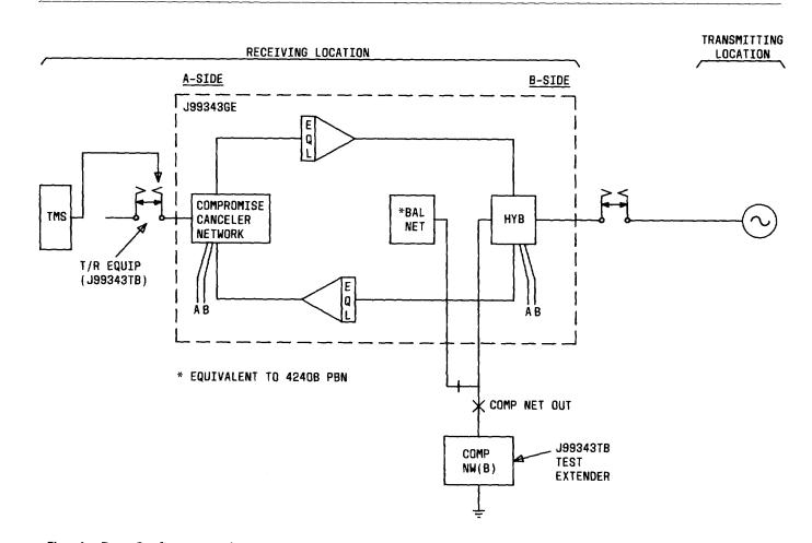
Fig. 4—Test Configuration for Frequency Response Measurements of the J99343GE Combined Function Unit
