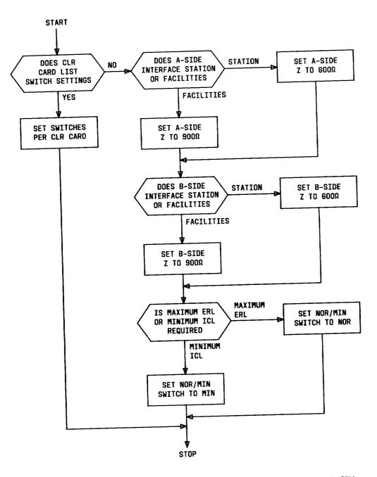
Fig. 3—Typical Switch Setting Decision Process for the J99343JA 2-W PLAR CFU
