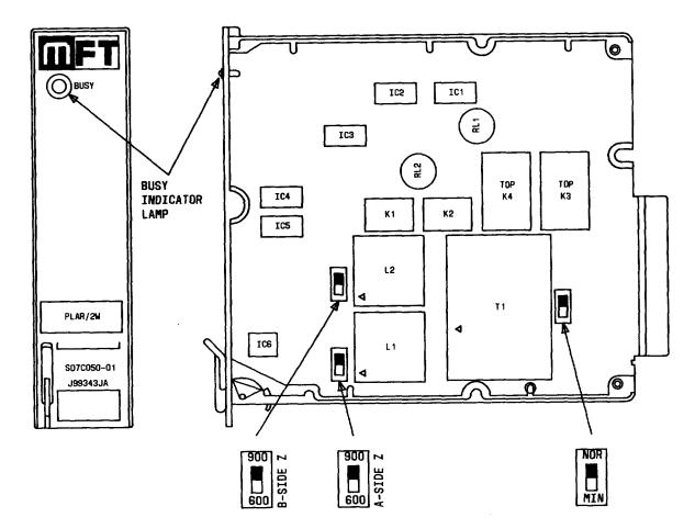
Fig. 1-J99343JA 2-W PLAR CFU-Switch Layout
