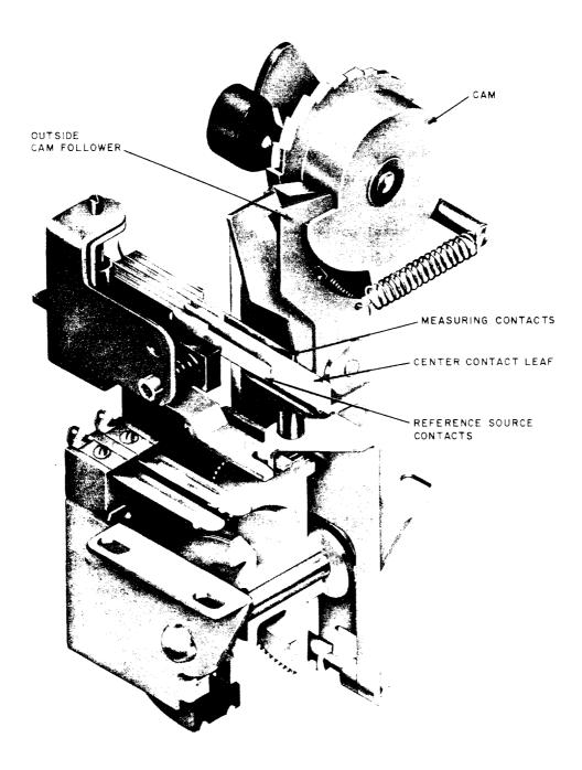
Fig. 1 — Indicator-Recorder Standardizer Assembly
