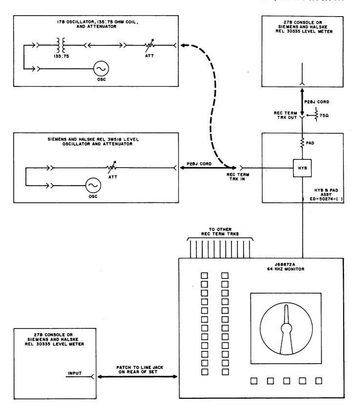
Fig. 2 — Check of Receiving Terminal Trunk for Through Transmission and Transmission to the J68872A Line Pilot Monitor Equipment
