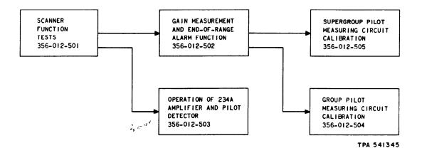
Fig. 1—J68858 Scanner and Test and Alarm Circuit—Testing Flow Chart
