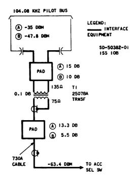
Fig. 2—104.08 kHz Pilot Bus Access Circuit (L600 Configuration)
