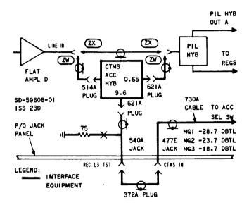
Fig. 5-L3 Receiving Access Circuit
