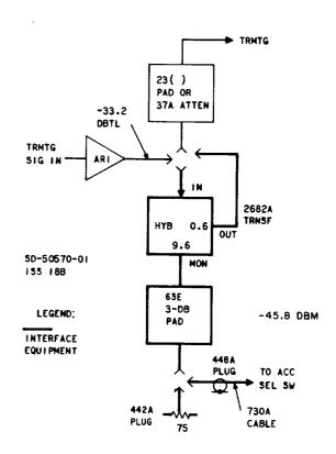
Fig. 2—3A WLEL Transmitting Access Circuit (for TD-2, TD-3, and TH-3)
