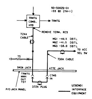
Fig. 4—TH-1 Transmitting Access Circuit
