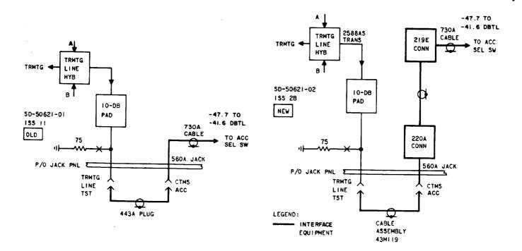
Fig. 8—L4 Transmitting Access Circuit
