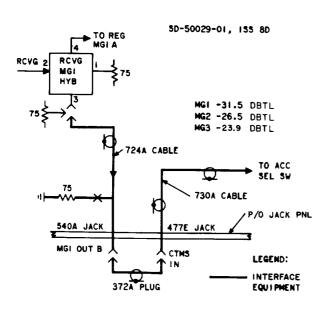
Fig. 3—TH-1 Receiving Access Circuit
