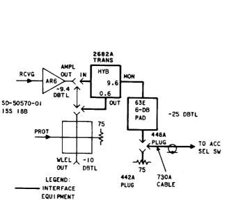
Fig. 1—3A WLEL Receiving Access Circuit (for TD-2, TD-3, and TH-3)
