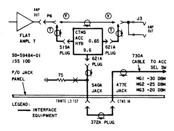
Fig. 6—L3 Transmitting Access Circuit
