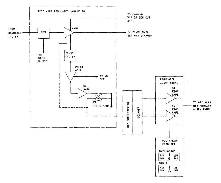
Fig. 4—Receiving Regulated Amplifier Gain and Alarm Circuits
