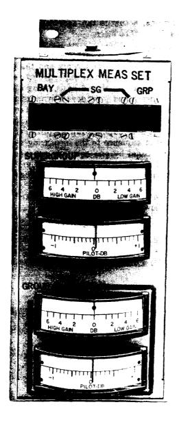
Fig. 2—Multiplex Measuring Set Meter Display
