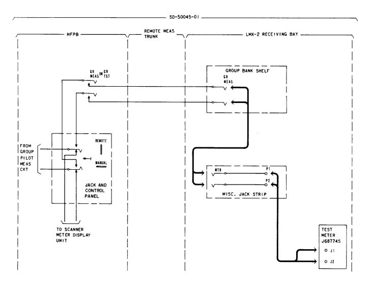
Fig. 9-Group Gain Remote Measuring Circuit
