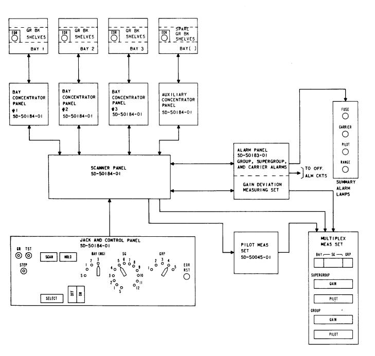
Fig. 1—Scanner and Test and Alarm Circuits—Block Diagram
