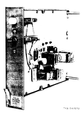
Fig. 9—J99335YA Tone Generator and Transfer Unit
