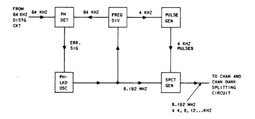
Fig. 5—Carrier Supply—Frequency Generating Circuit
