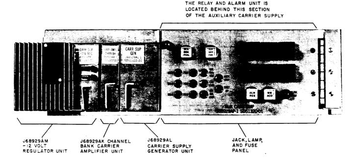
Fig. 2-\$A6 Auxiliary Carrier Supply\$
