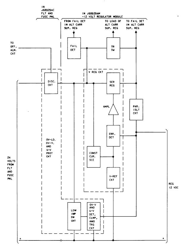
Fig. 6-\$J68929AM - 12 Volt Regulator-Block Diagram\$
