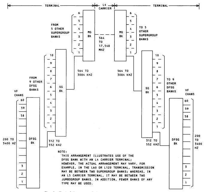
Fig. 2—Typical Function of the DFSG Bank in the L-Type Terminal
