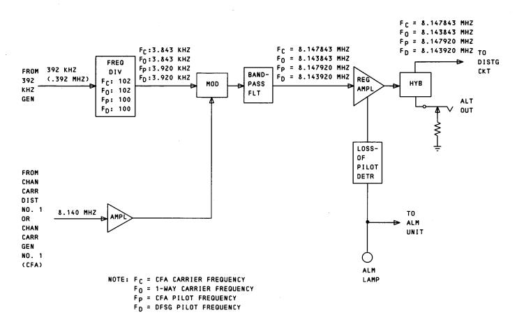
Fig. 14—CFA Carrier, One-Way Carrier, CFA Pilot, or DFSG Pilot Generator—Block Diagram
