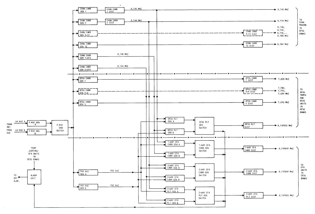
Fig. 9—DFSG-Bank Carrier Supply—Block Diagram
