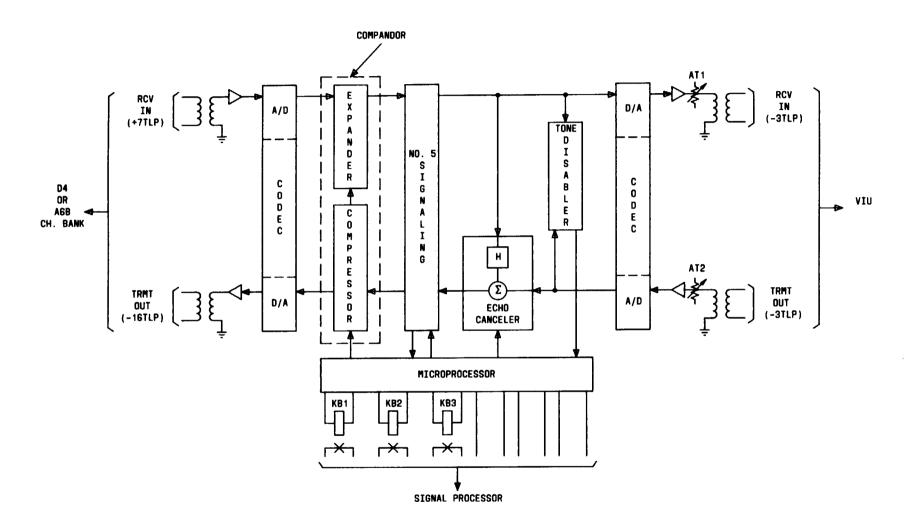
Fig. 2—J60110AA-1 Transceiver Block Diagram
