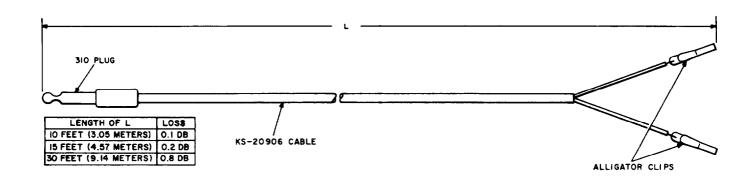
Fig. 11-Method of Constructing Special Cord\$
