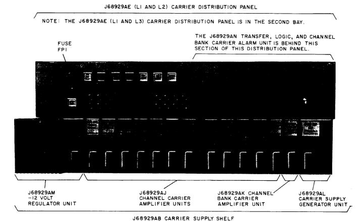
Fig. 3—A6 Carrier Supply and Distribution Panel
