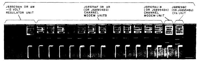
\* IF THE SHELF DOES NOT PROVIDE FOR CFA, THE J68929AG CHANNEL BANK MODEM MAY BE USED.
