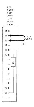
Fig. 21—Connections—Loss-of-Sync-Signal Test—Unprotected Carrier Supply
