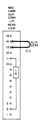
Fig. 14—Connections—Loss-of-Sync-Signal Test—Regular Carrier Supply
