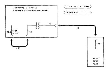
Fig. 7—Patching Diagram—Channel-Bank-Carrier Test—Regular Carrier Supply
