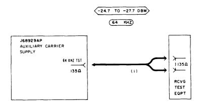
Fig. 10—Patching Diagram—Sync-Frequency Test—Auxiliary Carrier Supply
