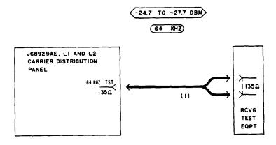
Fig. 4—Patching Diagram—Sync-Frequency Test—Regular Carrier Supply
