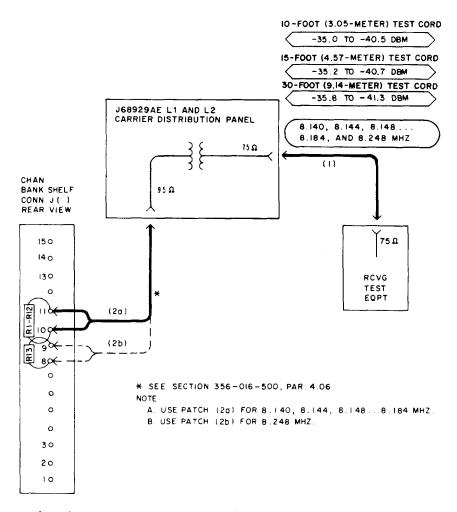
Fig. 13—PPatching Diagram—Carrier-Distribution Test—Auxiliary Carrier Supply
