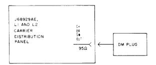
Fig. 23—Connections—Loss-of-Channel-Bank-Carrier Test—Unprotected Carrier Supply
