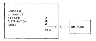
Fig. 24—Connections—Loss-of-Channel-Carriers Test— Unprotected Carrier Supply
