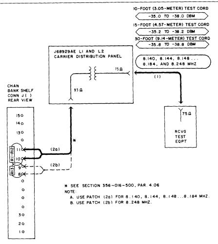
Fig. 9-Patching Diagram-Carrier-Distribution Test-Regular Carrier Supply
