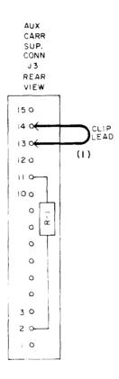
Fig. 19—Connections—Loss-of-Sync-Signal Test—Auxiliary Carrier Supply
