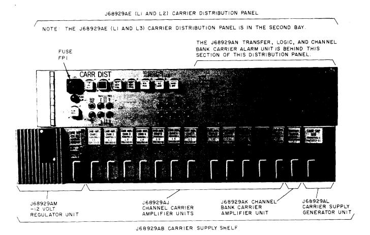
Fig. 1—A6 Carrier Supply and Distribution Panel—First Bay
