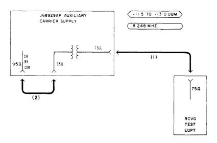
Fig. 12—Patching Diagram—Channel-Bank-Carrier Test—Auxiliary Carrier Supply
