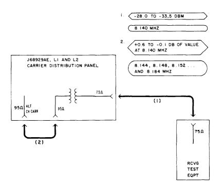
Fig. 6—Patching Diagram—Alternate (or Auxiliary) Channel-Carrier Test—At Regular Carrier Supply€
