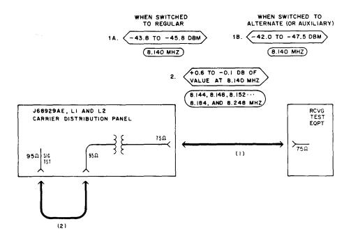
Fig. 5—PPatching Diagram—Carrier-Frequency Test—Regular Carrier Supply€
