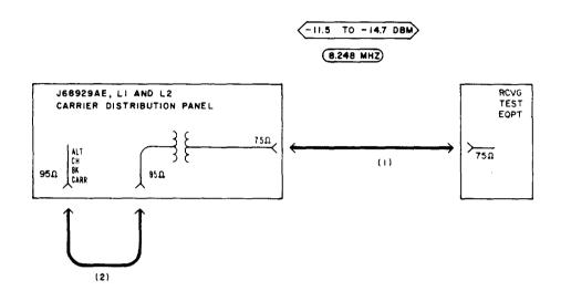
Fig. 8—Patching Diagram—Alternate (or Auxiliary) Channel-Bank-Carrier Test—At Regular Carrier Supply
