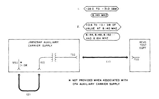
Fig. 11—PPatching Diagram—Carrier-Frequency Test—Auxiliary Carrier Supply
