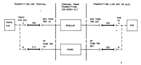
Fig. 2—Removing Regular Transmitting Trunks From Service—Patching Procedure
