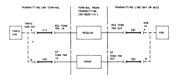
Fig. 3—Restoring Regular Transmitting Trunks to Service—Patching Procedure
