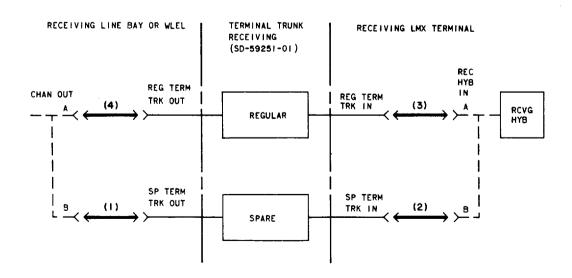
Fig. 4—Removing Regular Transmitting Trunks From Service—Patching Procedure
