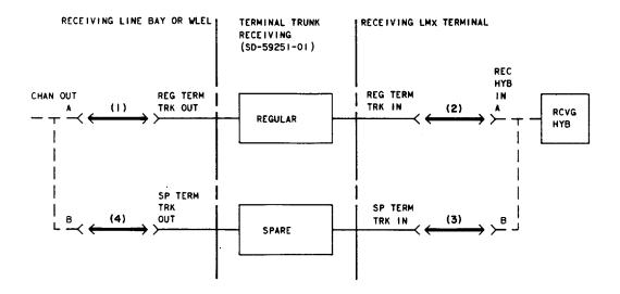
Fig. 5—Restoring Regular Receiving Trunks to Service—Patching Procedure
