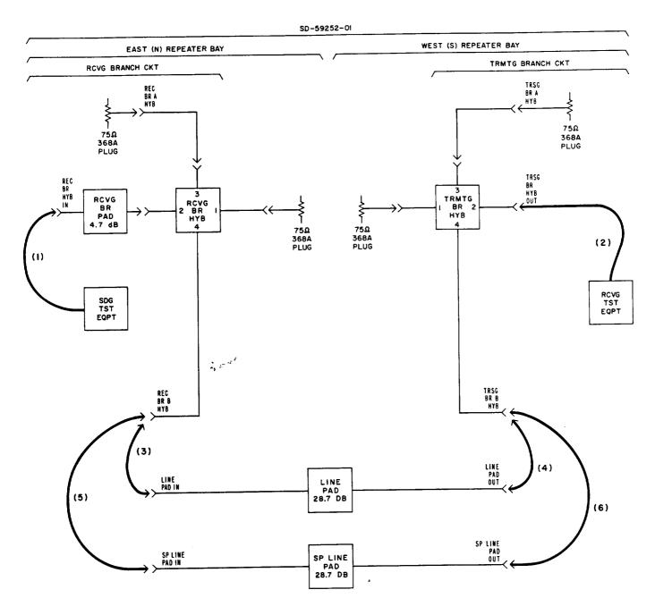
Fig. 2—Transmission Test of Line Pads
