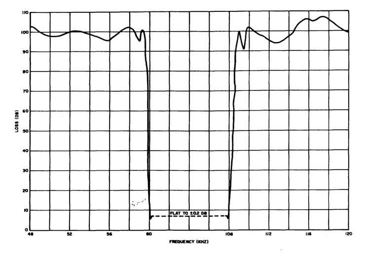
Fig. 3—4252() B3 Group Connector, Typical Loss Characteristic
