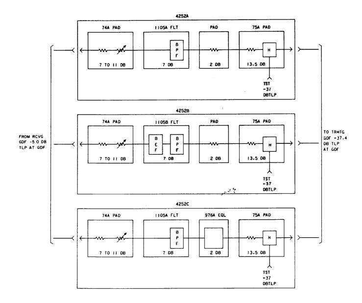
Fig. 2—B3 Group Connector, Simplified Schematic
