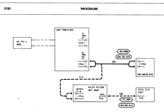
Fig. 4—Measurement of 104.08-kHz Pilot Signal Power
