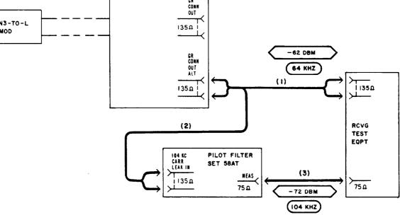
Fig. 3—Measurement of 64-kHz and 104-kHz Carrier Signal Power
