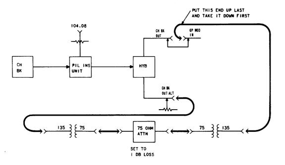
Fig. 2—Test Setup to Verify Through-Pilot Operation
