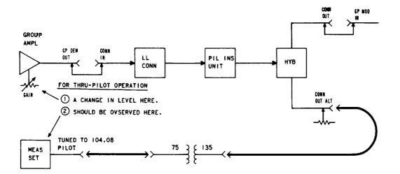
Fig. 3—Test Setup to Locate Pilot Block and Reinsert Location
