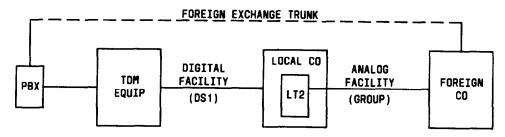
Fig. 5—Special Access #2 - Analog Office/Digital Station Signaling Applications
