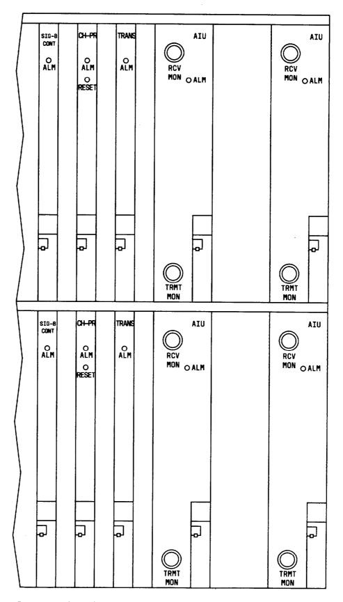
Fig. 8—48-Channel Module Equipped With Signaling and Echo Canceler Options (Extra Power Converter Required With Both Options) (Sheet 2 of 2)
