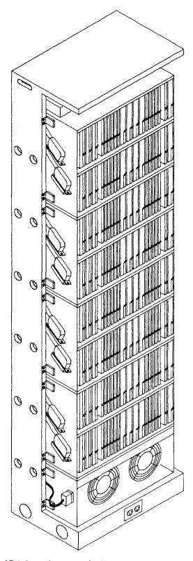
Fig. 6—J-68967A LT-2 Digital Transmultiplexer Bay Shown With Front Covers, Side Covers, and Fan Grill Removed
