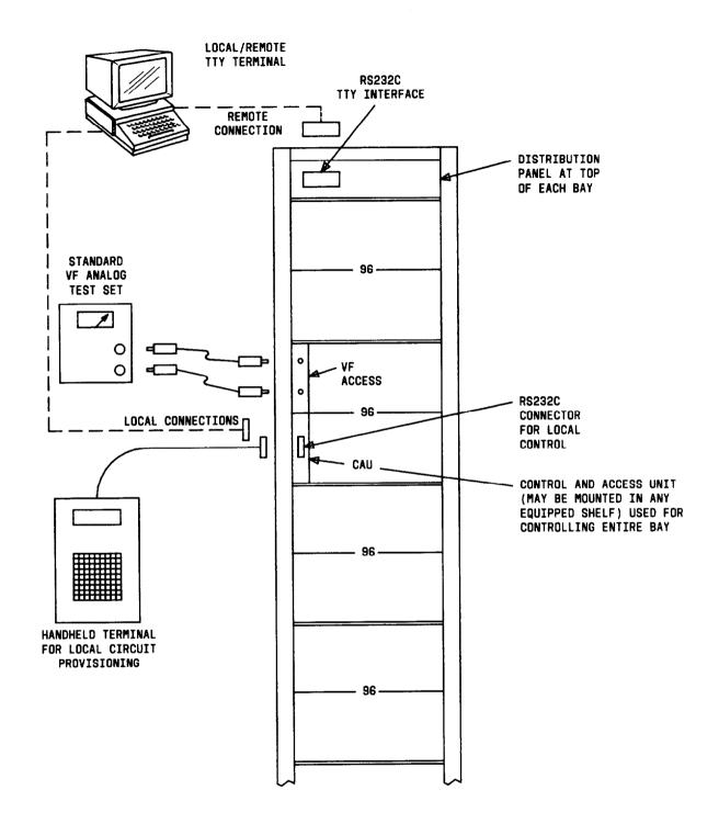
Fig. 1—LT-2 Bay Showing Local/Remote Maintenance Provisioning Arrangements
