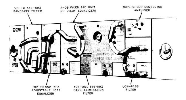
Fig. 9—J68858 C2B Supergroup Connector with Loss Equalizer and Pad Modules
