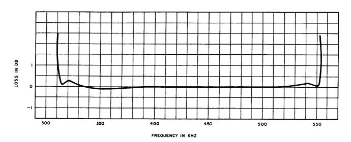
Fig. 11—C2 Supergroup Connector—Typical Loss Characteristic
