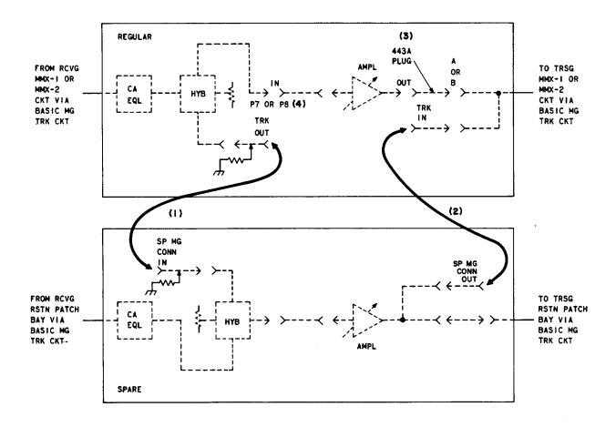
Fig. 3—Removing Regular Equipment From Service—Patching Procedure
