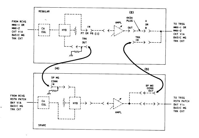
Fig. 6—Restoring Regular Equipment to Service—Patching Procedure
