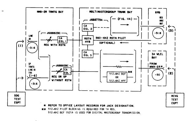
Fig. 1— ITransmitting Regular or Spare Radio Trunk Without Mastergroup Branching
