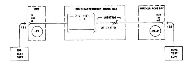
Fig. 4—Receiving Spare Mastergroup Bank Restoration Trunk
