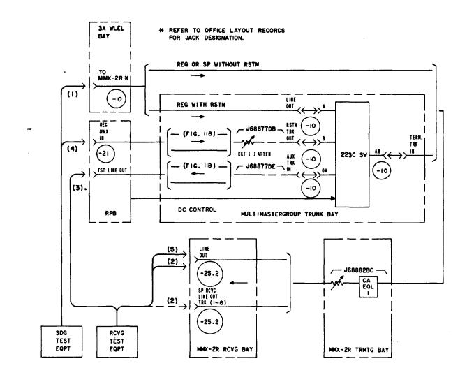
Fig. 2—Receiving Regular or Spare Radio Trunk Without Mastergroup Branching
