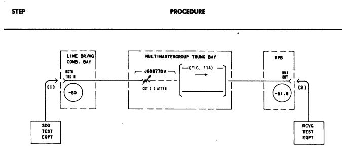
Fig. 7—Transmitting Restoration Trunk for Mastergroup Branching
