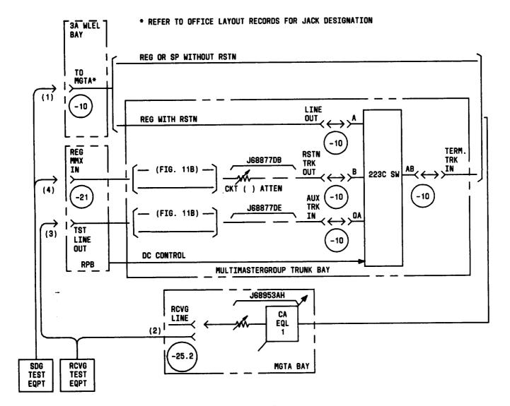
Fig. 10---- Receiving Trunks for MGTA\$
