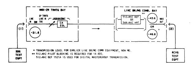
Fig. 5—Transmitting Regular or Spare Radio Trunk for Mastergroup Branching
