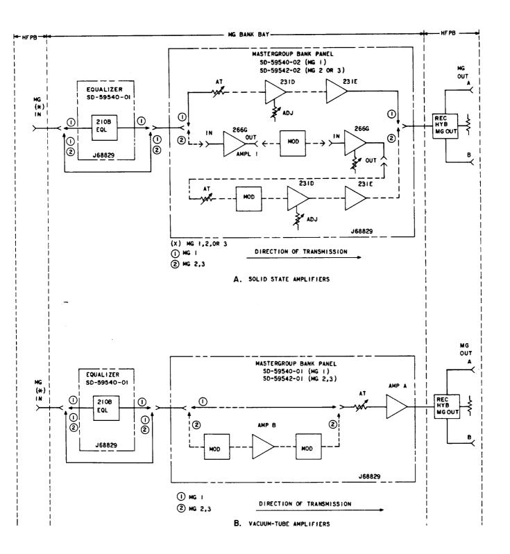
Fig. 3—Receiving Mastergroup Bank Circuit
