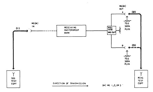
Fig. 1—Testing Arrangement
