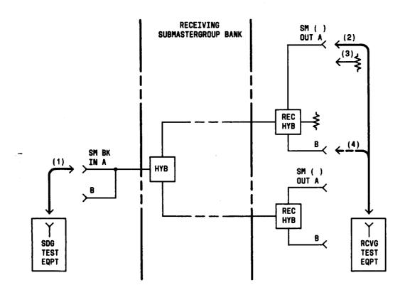
Fig. 3—Receiving Submastergroup Bank Testing Arrangement
