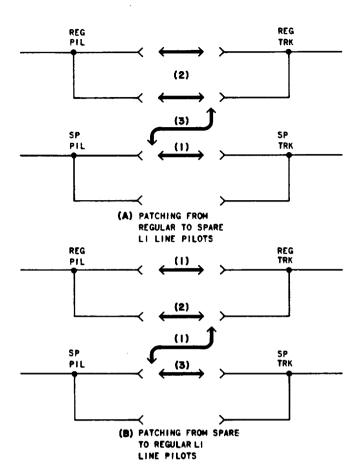
Fig. 1—L1 Line Pilot Switching—Patching Procedures
