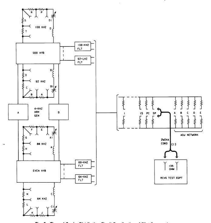
Fig. 2—Channel Carrier Distribution Circuit-Equalization of Pilot Frequencies
