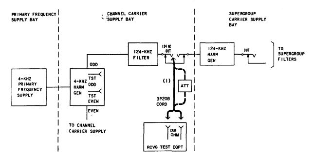
Fig. 2---Supergroup Carrier Supply---Measurement of 124-kHz Filter Output Power
