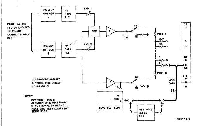
Fig. 2—Supergroup Carrier Supply—Measurement of Distribution Bus Power
